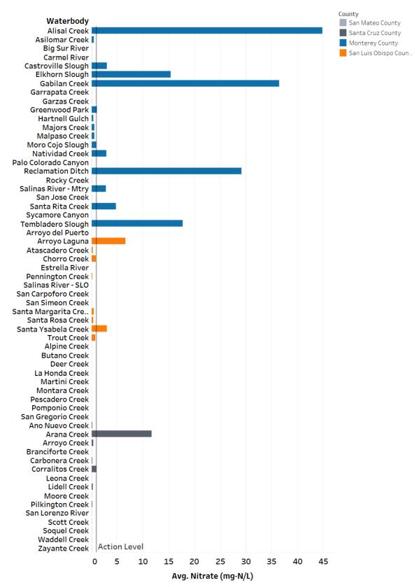
Figure 8. Average nitrate concentrations for each waterbody monitored. Waterbodies with more than one site have averaged results. Waterbodies are separated by county and the Action Level is indicated by the gray line.
