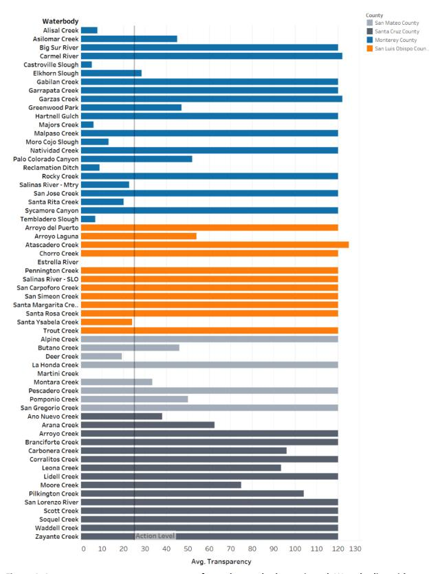
Figure 4. Average transparency measurements for each waterbody monitored. Waterbodies with more than one site have averaged results. Waterbodies are separated by county and the Action Level is indicated by the gray line.
