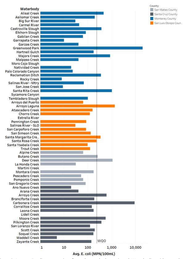
Figure 6. Average *E. coli* concentrations for each waterbody monitored. Waterbodies with more than one site have averaged results. Waterbodies are separated by county and the WQO is indicated by the gray line.
