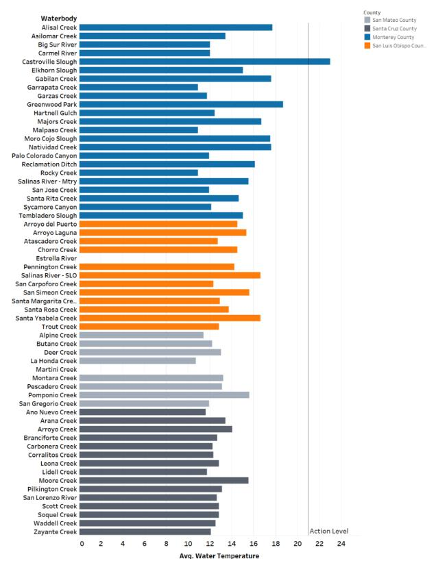
Figure 5. Average water temperature measurements for each waterbody monitored. Waterbodies with more than one site have averaged results. Waterbodies are separated by county and the Action Level is indicated by the gray line.
